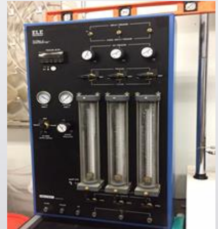
Figure 15: Tri-flex 2 Master Control Panel
